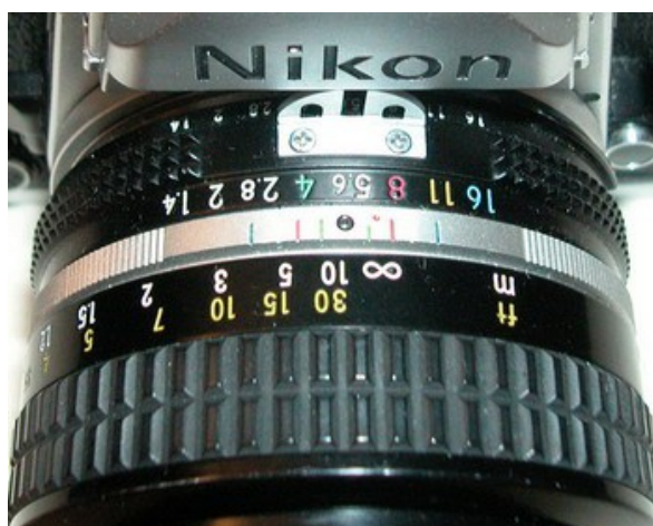
The lens is focused at infinity for IR photography (tiny red dot aligned with the ∞ symbol)
