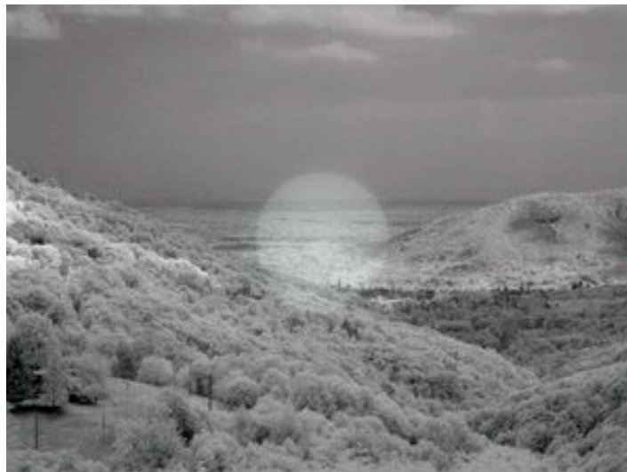
Hot-spot in a Nikon Coolpix E5000 with Hoya R72 IR filter (AF Auto t: 1/2s f:4,5 400ISO Zoom 21,4mm)
