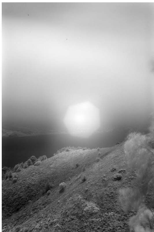
Hot-spot in a Canon 1DsMkII with IR B&W filter. Nikon 55mm/1.2 AIS lens. Similar behavior also occurs when using a Canon 16-35mm/2.8 USM L zoom and many other Canon 'L' lenses.
