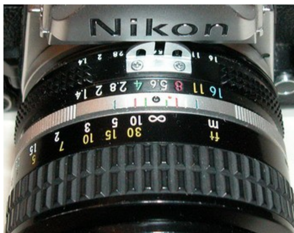
The lens is focused at infinity and in visible light (black dot aligned with the ∞ symbol)
