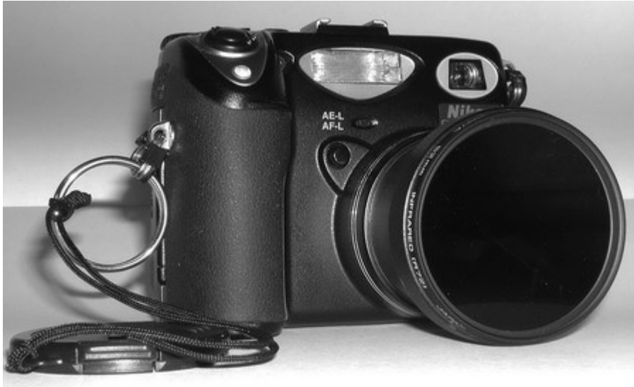
High-end digital point-and-shoot. The optical viewfinder (top right) allows us to frame the picture and shoot even though an IR filter has been mounted on the lens.
