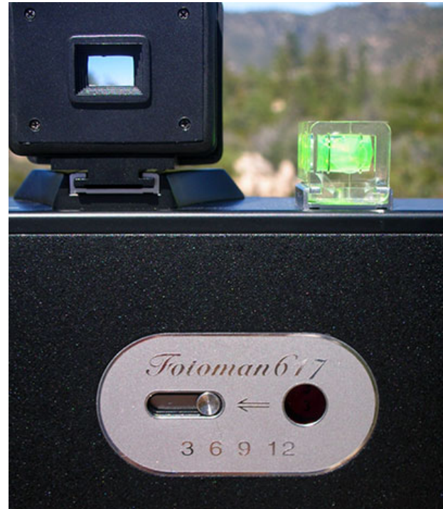
Figure 2: The rear red glass window. The arrow points in the direction of film winding and the engraved numbers are an invaluable memorandum during field operation.
